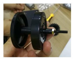
2.Put the gasket on the hole of the chassis, install the bearing wheel into the chassis.
