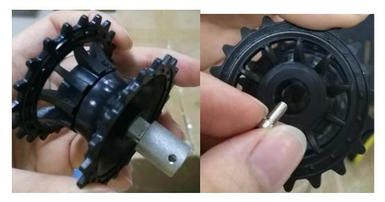
5. Install the driving wheel into the motor, lock it with top silk.
