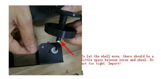
Install the gasket in another part, lock with M4 nut, Pls note that Do not tighten too much the bearing wheel.
