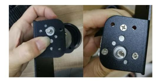
4.Install the driving wheel: Firstly install the connector into the driving wheel, use the wrench to install the M3\*8 hexagon screws into driving wheel to lock with the connector.
