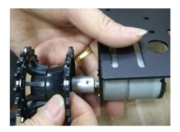
Note: The hole in the connector must be aligned with the flat end of the motor shaft, and the connector is stuck at the position of the arrow as the below picture showed.
