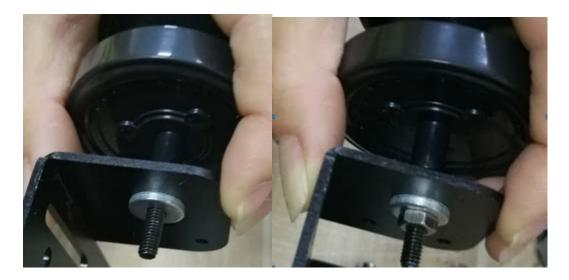
3.Install the motor into the chassis, lock it with 3pcs M3\*6mm flat haed screws.
